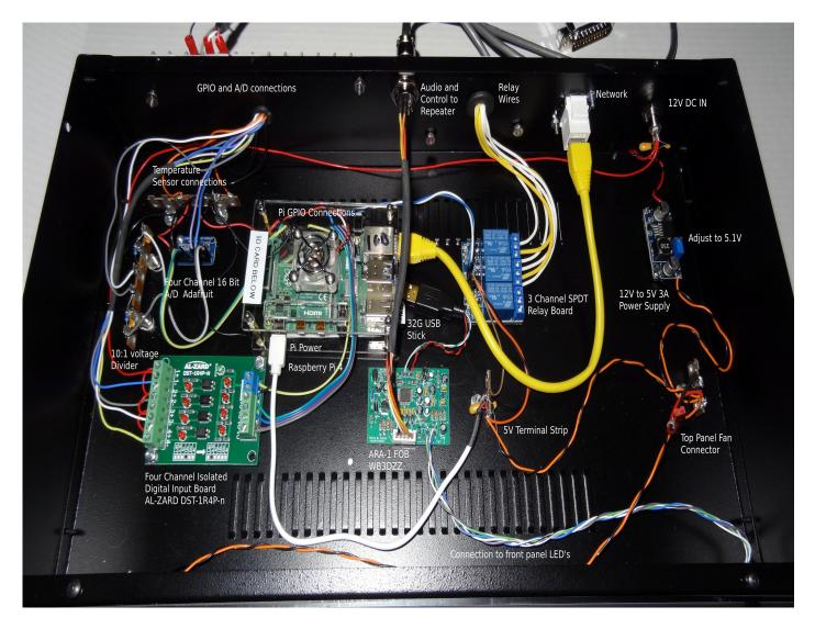
The controller is powered by 12v at the upper right through a barrel connector. This feeds to a 12v to 5V 3A power converter which supplies power for the majority of the components.
