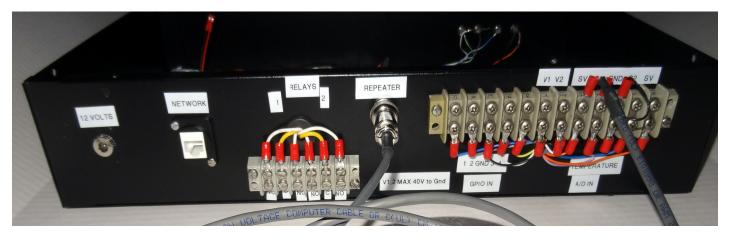
12V power is supplied via a barrel connector shown at the left. Maximum current draw is about 2A
