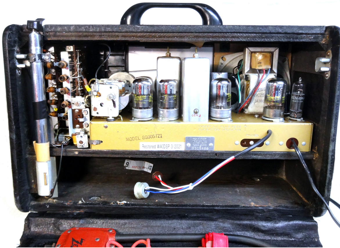
Chassis re-installed in the cabinet
