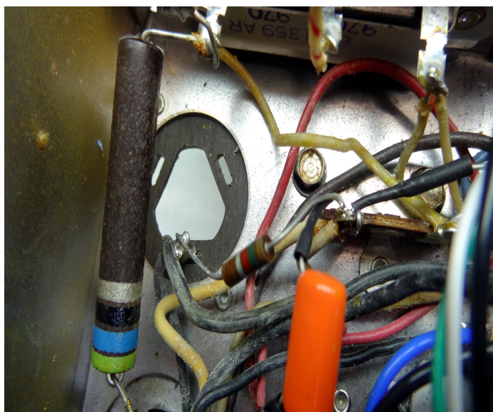
40/20/10uf Electrolytic removed
