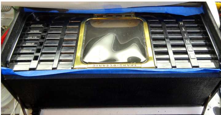
Carefully mask areas you do not want painted with the black leather dye. Cover the entire dial area also to avoid accidents.
